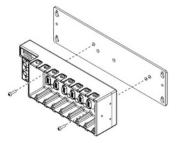
Use panel mount kits to mount your system in an enclosure or panel. The accessory kit for cDAQ chassis is a metal plate with pre-drilled holes so you can mount your system with tool access from the front.
