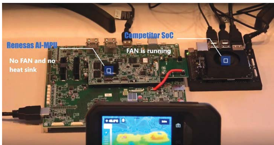
Figure 12: Comparison of Heat Generation between a Fanless DRP-AI Test Board and a GPU with Fan
